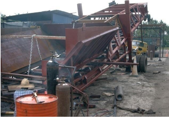
7' feet belt width Hopper Conveyor (own design)
