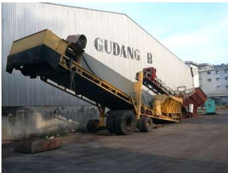
5' feet belt width x 50' feet long Deck Conveyor (own design)
