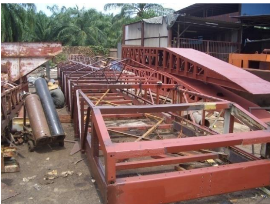
5' feet belt width x 50' feet long Deck Conveyor (own design)
