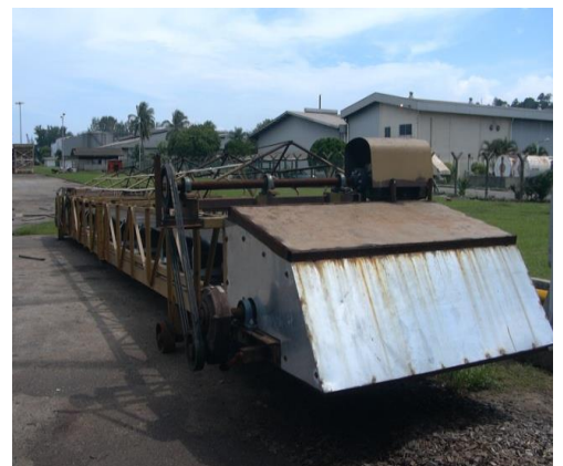
5' feet belt width x 50' feet long Deck Conveyor (own design)
